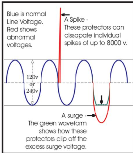
The ZAP-PRO protectors are *plug-in* devices that intercept most voltage problems **BEFORE** they get a chance to do any damage to the circuit boards or components. The chart at left shows what AC waveforms look like on an oscilloscope, and also shows what some damaging transients might look like.
